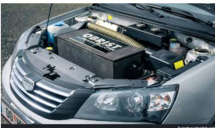
**First approach:** I open the hood and my eyes fall on the first of two black boxes installed in the car: The encapsulated front unit holds the two-cylinder engine and generator. The unit itself is built only 188 millimeters wide and it is probably well recognizable to laymen, how much space remains free, if instead of the original burner, this "Obrist-box" is used.
