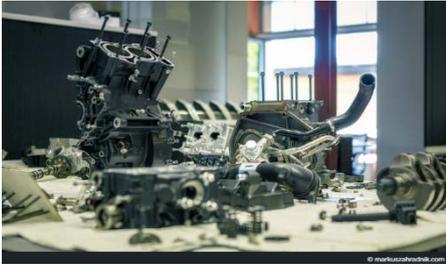
**From 4 make 2:** Conceived, adapted, developed and built in-house: the small one-liter unit that feeds the batteries of the HyperHybrid via a generator.
