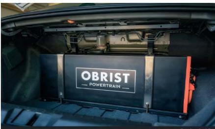
**The battery:** Depending on the capacity, current E-car batteries weigh up to 800 kilograms and therefore need a lot of space, no matter where they are placed in the car. The extremely compact 11kWh Obrist solution, on the other hand, weighs only 112 kilograms and takes little away from the trunk. Mind you: this is a bodywork that was not intended for such magic in series. You can't imagine how easy the system could be transferred to any vehicle.
