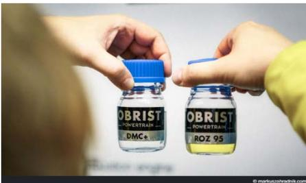
**Miracle Fuel DMC+:** Frank Obrist: "We are the first company in the world to have CO<sub>2</sub> neutral fuel in house." DMC+ is a 115-octane gasoline and diesel replacement that does not smoke when burned. If the suggestively-good-smelling fuel would prevail across the board, zero emissions would be reached. Disadvantage: To replace the energy density of 1 liter of gasoline, you need 2 liters of DMC+; that is, twice as large tanks.
